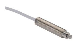
Metrol limit switch, precision touch, 8mm diameter, threaded, 0.75mm pitch, 43.5mm length, 3mm radius head, stainless steel, 3.5mm plunger, 1N contact force, (1) N.O. contact(s), 9.8ft/3m cable length, pigtail.
