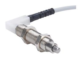
Metrol limit switch, precision touch, 8mm diameter, threaded, 0.75mm pitch, 49.5mm length, 1.5mm radius head, stainless steel, 2mm plunger, 1N contact force, N.O. contact(s), 9.8ft/3m cable length, 90 degree exit, pigtail.
