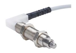
Metrol limit switch, precision touch, 8mm diameter, threaded, 0.75mm pitch, 49.5mm length, 1.5mm radius head, stainless steel, 2mm plunger, 1N contact force, (1) N.O. contact(s), 9.8ft/3m cable length, 90 degree exit, pigtail.
