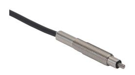
Metrol limit switch, precision touch, 6mm diameter, threaded, 0.75mm pitch, 42mm length, 1.5mm radius head, stainless steel, 2mm plunger, 1N contact force, (1) N.C. contact(s), 9.8ft/3m cable length, pigtail.
