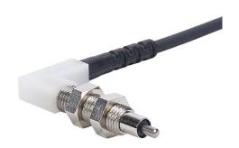
Metrol limit switch, precision touch, 6mm diameter, threaded, 0.75mm pitch, 37mm length, 1.5mm radius head, stainless steel, 2mm plunger, 1N contact force, N.C. contact(s), 9.8ft/3m cable length, 90 degree exit, pigtail.
