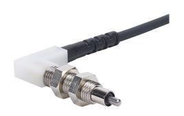
Metrol limit switch, precision touch, 6mm diameter, threaded, 0.75mm pitch, 37mm length, 1.5mm radius head, stainless steel, 2mm plunger, 1N contact force, (1) N.C. contact(s), 9.8ft/3m cable length, 90 degree exit, pigtail.
