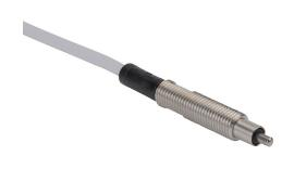
Metrol limit switch, precision touch, 6mm diameter, threaded, 0.75mm pitch, 42mm length, 1.5mm radius head, stainless steel, 2mm plunger, 1N contact force, (1) N.O. contact(s), 9.8ft/3m cable length, pigtail.
