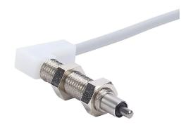
Metrol limit switch, precision touch, 6mm diameter, threaded, 0.75mm pitch, 40mm length, 1.5mm radius head, stainless steel, 2mm plunger, 1N contact force, (1) N.O. contact(s), 9.8ft/3m cable length, 90 degree exit, pigtail.
