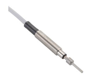
Metrol limit switch, precision touch, 6mm diameter, threaded, 0.75mm pitch, 55.5mm length, 1.5mm flat head, stainless steel, needle plunger, 1N contact force, (1) N.O. contact(s), 9.8ft/3m cable length, pigtail.
