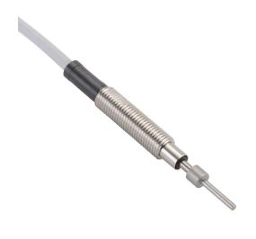
Metrol limit switch, precision touch, 6mm diameter, threaded, 0.75mm pitch, 55.5mm length, 1.5mm flat head, stainless steel, needle plunger, 1N contact force, N.O. contact(s), 9.8ft/3m cable length, pigtail.
