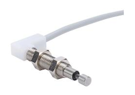
Metrol limit switch, precision touch, 6mm diameter, threaded, 0.75mm pitch, 40mm length, 4.5mm flat head, stainless steel, 2mm plunger, 1N contact force, (1) N.O. contact(s), 9.8ft/3m cable length, 90 degree exit, pigtail.
