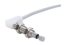
Metrol limit switch, precision touch, 6mm diameter, threaded, 0.75mm pitch, 40mm length, 4.5mm flat head, stainless steel, 2mm plunger, 1N contact force, N.O. contact(s), 9.8ft/3m cable length, 90 degree exit, pigtail.
