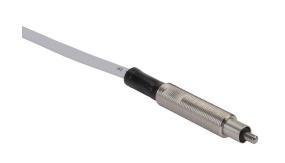
Metrol limit switch, precision touch, 6mm diameter, threaded, 0.5mm pitch, 42mm length, 1.5mm radius head, stainless steel, 2mm plunger, 1N contact force, (1) N.O. contact(s), 9.8ft/3m cable length, pigtail.
