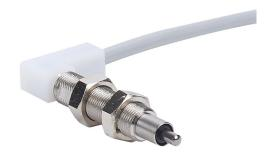
Metrol limit switch, precision touch, 6mm diameter, threaded, 0.5mm pitch, 40mm length, 1.5mm radius head, stainless steel, 2mm plunger, 1N contact force, (1) N.O. contact(s), 9.8ft/3m cable length, 90 degree exit, pigtail.
