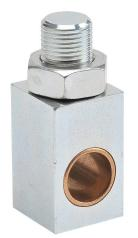
NITRA rod eye, 5/8-18 UNF thread, zinc plated steel. For use with C-series cylinders. Bronze pivot bushing and nut included.
