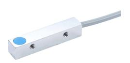
AutomationDirect inductive proximity sensor, rectangular,  $8 \times 8 \times 40$ mm body, nickel-plated brass housing, PNP, N.O. output, 3mm sensing distance, semi-flush, 1 kHz switching frequency, IP67, pigtail.
