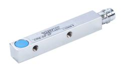
AutomationDirect inductive proximity sensor, rectangular, 8 x 8 x 59mm body, nickel-plated brass housing, PNP, N.O. output, 2mm sensing distance, flush, 1 kHz switching frequency, IP67, 3-pin M8 quick-disconnect.
