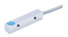
AutomationDirect inductive proximity sensor, rectangular, 8 x 8 x 40mm body, nickel-plated brass housing, PNP, N.O. output, 2mm sensing distance, flush, 1 kHz switching frequency, IP67, pigtail.
