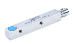
AutomationDirect inductive proximity sensor, rectangular, 8 x 8 x 59mm body, nickel-plated brass housing, PNP, N.O. output, 1.5mm sensing distance, flush, 1 kHz switching frequency, IP67, 3-pin M8 quick-disconnect.
