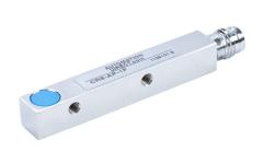
AutomationDirect inductive proximity sensor, rectangular, 8 x 8 x 59mm body, nickel-plated brass housing, PNP, N.O. output, 1.5mm sensing distance, flush, 1 kHz switching frequency, IP67, 3-pin M8 quick-disconnect.
