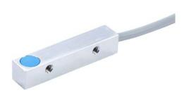
AutomationDirect inductive proximity sensor, rectangular, 8 x 8 x 40mm body, nickel-plated brass housing, PNP, N.O. output, 1.5mm sensing distance, flush, 1 kHz switching frequency, IP67, pigtail.
