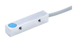
AutomationDirect inductive proximity sensor, rectangular,  $8 \times 8 \times 40$ mm body, nickel-plated brass housing, PNP, N.O. output, 1.5mm sensing distance, flush, 1 kHz switching frequency, IP67, pigtail.
