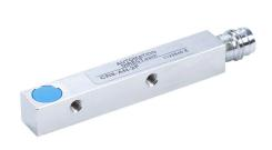
AutomationDirect inductive proximity sensor, rectangular, 8 x 8 x 59mm body, nickel-plated brass housing, NPN, N.O. output, 2mm sensing distance, flush, 1 kHz switching frequency, IP67, 3-pin M8 quick-disconnect.
