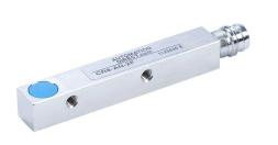
AutomationDirect inductive proximity sensor, rectangular, 8 x 8 x 59mm body, nickel-plated brass housing, NPN, N.O. output, 2mm sensing distance, flush, 1 kHz switching frequency, IP67, 3-pin M8 quick-disconnect.
