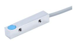
AutomationDirect inductive proximity sensor, rectangular, 8 x 8 x 40mm body, nickel-plated brass housing, NPN, N.O. output, 2mm sensing distance, flush, 1 kHz switching frequency, IP67, pigtail.
