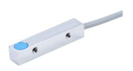
AutomationDirect inductive proximity sensor, rectangular, 8 x 8 x 40mm body, nickel-plated brass housing, NPN, N.O. output, 2mm sensing distance, flush, 1 kHz switching frequency, IP67, pigtail.
