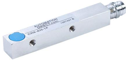
AutomationDirect inductive proximity sensor, rectangular, 8 x 8 x 59mm body, nickel-plated brass housing, NPN, N.O. output, 1.5mm sensing distance, flush, 1 kHz switching frequency, IP67, 3-pin M8 quick-disconnect.
