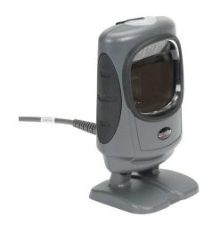
Code barcode scanner, 1D and 2D, imager, corded, USB, general duty, 1280 x 960 optical resolution. 6ft USB cable included.
