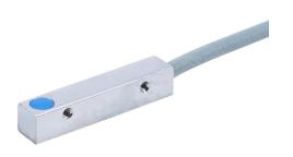
AutomationDirect inductive proximity sensor, rectangular,  $5 \times 5 \times 25 \text{mm}$  body, nickel-plated brass housing, PNP, N.O. output, 1.5mm sensing distance, flush, 3 kHz switching frequency, IP67, 3-pin M8 quick-disconnect.
