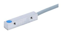
AutomationDirect inductive proximity sensor, rectangular,  $5 \times 5 \times 25$ mm body, nickel-plated brass housing, PNP, N.O. output, 1.5mm sensing distance, flush, 3 kHz switching frequency, IP67, 3-pin M8 quick-disconnect.
