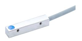
AutomationDirect inductive proximity sensor, rectangular,  $5 \times 5 \times 25 \text{mm}$  body, nickel-plated brass housing, PNP, N.O. output, 0.8mm sensing distance, flush, 5 kHz switching frequency, IP67, 3-pin M8 quick-disconnect.
