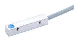
AutomationDirect inductive proximity sensor, rectangular, 5 x 5 x 25mm body, nickel-plated brass housing, PNP, N.O. output, 0.8mm sensing distance, flush, 5 kHz switching frequency, IP67, 3-pin M8 quick-disconnect.
