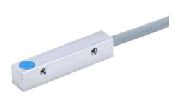
AutomationDirect inductive proximity sensor, rectangular,  $5 \times 5 \times 25 \text{mm}$  body, nickel-plated brass housing, PNP, N.O. output, 0.8mm sensing distance, flush, 5 kHz switching frequency, IP67, pigtail.
