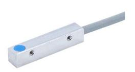
AutomationDirect inductive proximity sensor, rectangular, 5  $\times$  5  $\times$  25mm body, nickel-plated brass housing, PNP, N.O. output, 0.8mm sensing distance, flush, 5 kHz switching frequency, IP67, pigtail.
