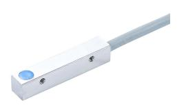
AutomationDirect inductive proximity sensor, rectangular,  $5 \times 5 \times 25 \text{mm}$  body, nickel-plated brass housing, NPN, N.O. output, 1.5mm sensing distance, flush, 3 kHz switching frequency, IP67, 3-pin M8 quick-disconnect.
