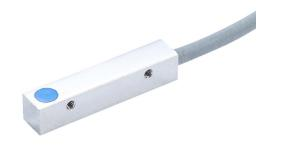
AutomationDirect inductive proximity sensor, rectangular, 5 x 5 x 25mm body, nickel-plated brass housing, NPN, N.O. output, 1.5mm sensing distance, flush, 3 kHz switching frequency, IP67, pigtail.
