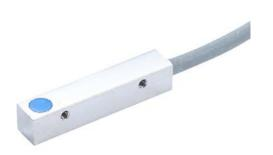
AutomationDirect inductive proximity sensor, rectangular,  $5 \times 25$  mm body, nickel-plated brass housing, NPN, N.O. output, 1.5mm sensing distance, flush, 3 kHz switching frequency, IP67, pigtail.
