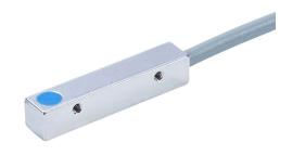
AutomationDirect inductive proximity sensor, rectangular, 5 x 5 x 25mm body, nickel-plated brass housing, NPN, N.O. output, 0.8mm sensing distance, flush, 5 kHz switching frequency, IP67, pigtail.
