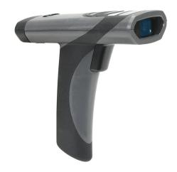
Code barcode scanner, 1D and 2D, imager, cordless, Bluetooth communication, USB, general duty, 1280 x 960 optical resolution. Removable battery, charging base station and 3ft USB cable included.
