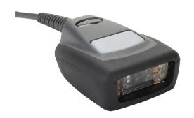
Code barcode scanner, 1D and 2D, imager, corded, USB, general duty, dual  $960 \times 640$  optical resolution. 6ft USB cable included.
