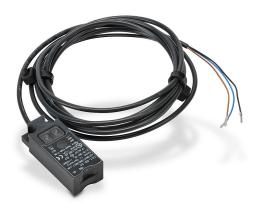
AutomationDirect capacitive proximity sensor, rectangular, 20 x 14 x 48mm body, polybutylene terephthalate housing, NPN/PNP, N.O./N.C. selectable output, 12mm sensing distance, non-flush, 10 Hz switching frequency, IP65 IP67, pigtail.
