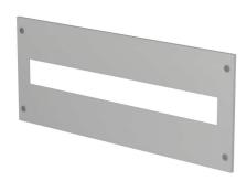
Quadritalia OK series modular cover, 200 x 600mm (HxW), 1 cutout, 47 x 430mm connector cutout(s), carbon steel, RAL 7035 light gray, powder coat finish. For use with TMKxx6 inner frame in 600mm width enclosures.
