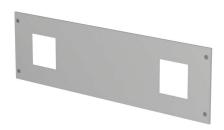
Quadritalia OK series modular cover, 200 x 800mm (HxW), 2 cutouts, 92 x 92mm connector cutout(s), carbon steel, RAL 7035 light gray, powder coat finish. For use with TMKxx8 inner frame in 800mm width enclosures.
