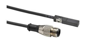
NITRA cylinder switch, square, PNP, N.O. output, 10-30 VDC operating voltage, LED indication, IP69K, 0.3m (1ft) cable with M12 connector, 5mm square T-slot mount, for position sensing.
