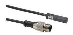
NITRA cylinder switch, square, PNP, N.O. output, 10-30 VDC operating voltage, LED indication, IP69K, 0.3m (1ft) cable with M12 connector, straight cable entry, 5mm square T-slot mount, for position sensing.
