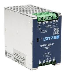
LUTZE CPS 3-phase series switching power supply, 24 VDC @ 40A/960W, 480 VAC nominal input, 3-phase, enclosed, aluminum housing, 35mm DIN rail mount, screw terminals.
