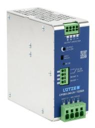
LUTZE CPS 3-phase series switching power supply, 24 VDC @ 10A/240W, 480 VAC nominal input, 3-phase, enclosed, aluminum housing, 35mm DIN rail mount, push terminals.
