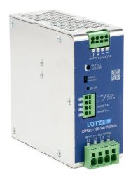
LUTZE CPS 3-phase series switching power supply, 24 VDC @ 5A/120W, 480 VAC nominal input, 3-phase, enclosed, aluminum housing, 35mm DIN rail mount, push terminals.
