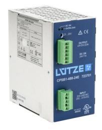
LUTZE CPS Eco series switching power supply, 24 VDC @ 20A/480W, 220 VAC nominal input, 1-phase, enclosed, aluminum housing, 35mm DIN rail mount, screw terminals.
