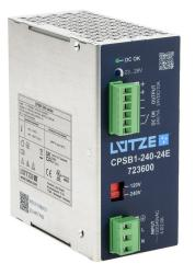
LUTZE CPS Eco series switching power supply, 24 VDC @ 10A/240W, 120/240 VAC nominal input, 1-phase, enclosed, aluminum housing, 35mm DIN rail mount, screw terminals.
