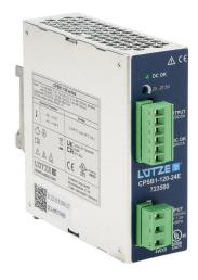
LUTZE CPS Eco series switching power supply, 24 VDC @ 5A/120W, 120 VAC nominal input, 1-phase, enclosed, aluminum housing, 35mm DIN rail mount, screw terminals.
