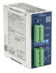
LUTZE CPS Universal series switching power supply, 24 VDC @ 10A/240W, 220/480 VAC nominal input, 1, 2 and 3-phase, enclosed, aluminum housing, 35mm DIN rail mount, screw terminals.
