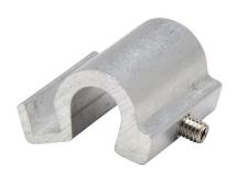
NITRA adapter bracket, for use with a 5mm square cylinder position switch and a 3/16 to 1/4in (5 to 7mm) diameter tie rod.
