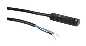
NITRA cylinder switch, rectangular, NPN, N.O. output, 5-28 VDC operating voltage, LED indication, 9.8ft (3.00m) 3-wire pigtail with wire leads, straight cable entry, 7.2 x 3.9mm T-slot mount, for position sensing.
