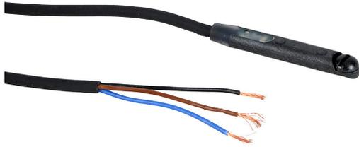
NITRA cylinder switch, rectangular, low profile, PNP, N.O. output, 5-28 VDC operating voltage, LED indication, 9.8ft (3.00m) 3-wire pigtail with wire leads, straight cable entry, 6.5 x 3.2mm T-slot mount, for position sensing.
