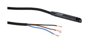
NITRA cylinder switch, rectangular, low profile, PNP, N.O. output, 5-28 VDC operating voltage, LED indication, 9.8ft (3.00m) 3-wire pigtail with wire leads, 6.5 x 3.2mm T-slot mount, for position sensing.
