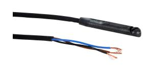
NITRA cylinder switch, rectangular, low profile, NPN, N.O. output, 5-28 VDC operating voltage, LED indication, 9.8ft (3.00m) 3-wire pigtail with wire leads, 6.5 x 3.2mm T-slot mount, for position sensing.
