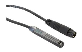
NITRA cylinder switch, round, PNP, N.O. output, 5-28 VDC operating voltage, LED indication, 0.5ft (0.15m) cable with 3-pin M8 snap-fit connector, straight cable entry, 1/4in round slot mount, for position sensing.
