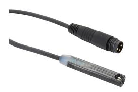
NITRA cylinder switch, round, NPN, N.O. output, 5-28 VDC operating voltage, LED indication, 0.5ft (0.15m) cable with 3-pin M8 snap-fit connector, straight cable entry, 1/4in round slot mount, for position sensing.
