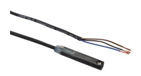
NITRA cylinder switch, round, NPN, N.O. output, 5-28 VDC operating voltage, LED indication, 9.8ft (3.00m) 3-wire pigtail with wire leads, straight cable entry, 1/4in round slot mount, for position sensing.
