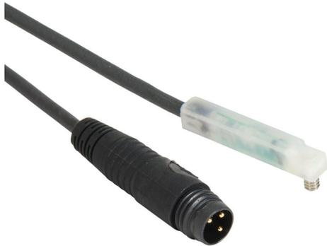
NITRA cylinder switch, square, PNP, N.O. output, 5-28 VDC operating voltage, LED indication, 0.5ft (0.15m) cable with 3-pin M8 snap-fit connector, straight cable entry, 4mm square T-slot mount, for position sensing.
