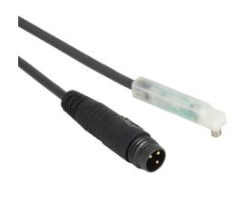
NITRA cylinder switch, square, PNP, N.O. output, 5-28 VDC operating voltage, LED indication, 0.5ft (0.15m) cable with 3-pin M8 snap-fit connector, straight cable entry, 4mm square T-slot mount, for position sensing.
