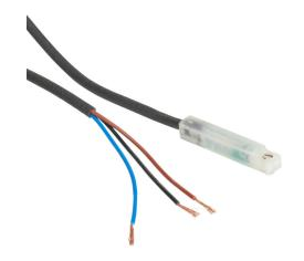
NITRA cylinder switch, square, PNP, N.O. output, 5-28 VDC operating voltage, LED indication, 9.8ft (3.00m) 3-wire pigtail with wire leads, straight cable entry, 4mm square T-slot mount, for position sensing.
