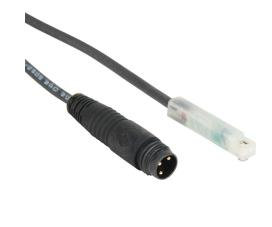
NITRA cylinder switch, square, NPN, N.O. output, 5-28 VDC operating voltage, LED indication, 0.5ft (0.15m) cable with 3-pin M8 snap-fit connector, straight cable entry, 4mm square T-slot mount, for position sensing.
