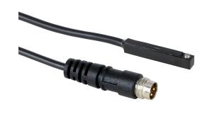
NITRA cylinder switch, square, NPN, N.O. output, 5-28 VDC operating voltage, LED indication, 0.5ft (0.15m) cable with 3-pin M8 snap-fit connector, 4mm square T-slot mount, for position sensing.
