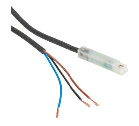
NITRA cylinder switch, square, NPN, N.O. output, 5-28 VDC operating voltage, LED indication, 9.8ft (3.00m) 3-wire pigtail with wire leads, straight cable entry, 4mm square T-slot mount, for position sensing.
